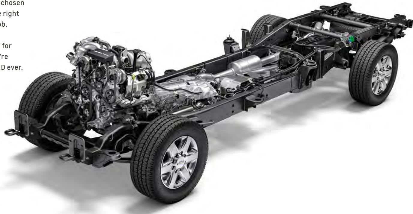
To create a solid structure that stands up to heavy-duty usage, we used a combination of **high-strength and ultra-high-strength steel** throughout the cab and frame.
