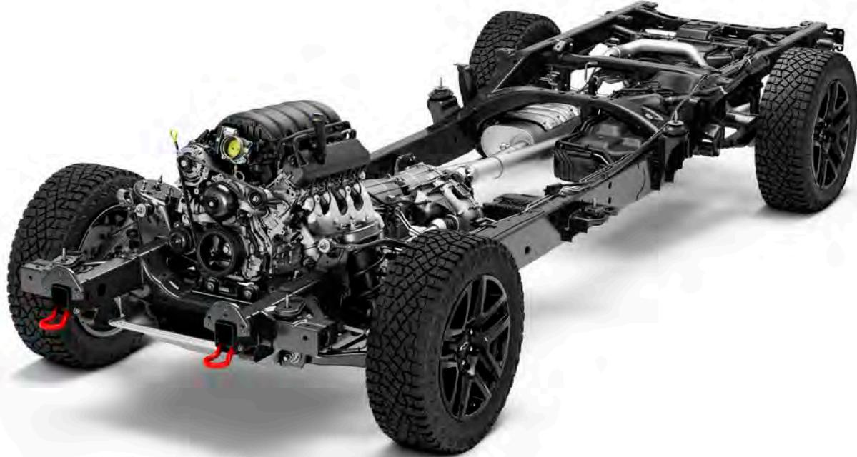
The **independent short/long arm front suspension** provides excellent wheel alignment, ride comfort and tunability with reduced weight. The live axle rear suspension includes 2-stage, semi-elliptic multileaf springs to strike a balance between payload management and ride quality.
